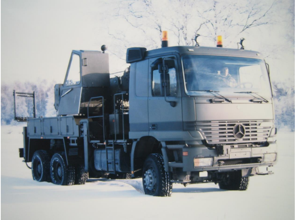
Mercedes-Benz Actros (6x6) trucks fitted with different recovery equipment. While the vehicle above represents a military wrecker with high cross-country performance to be noticed by the high ground clearance and crane, the vehicle below is designed for heavy recovery operations mostly on roads. The latter vehicle is equipped with a towing device at the rear and lacks the heavy crane.
