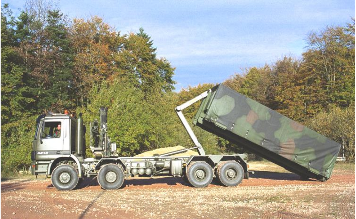
This Mercedes-Benz truck 3243A (8x8) MULTI is equipped with a modern load-handling system and an auxiliary crane.
