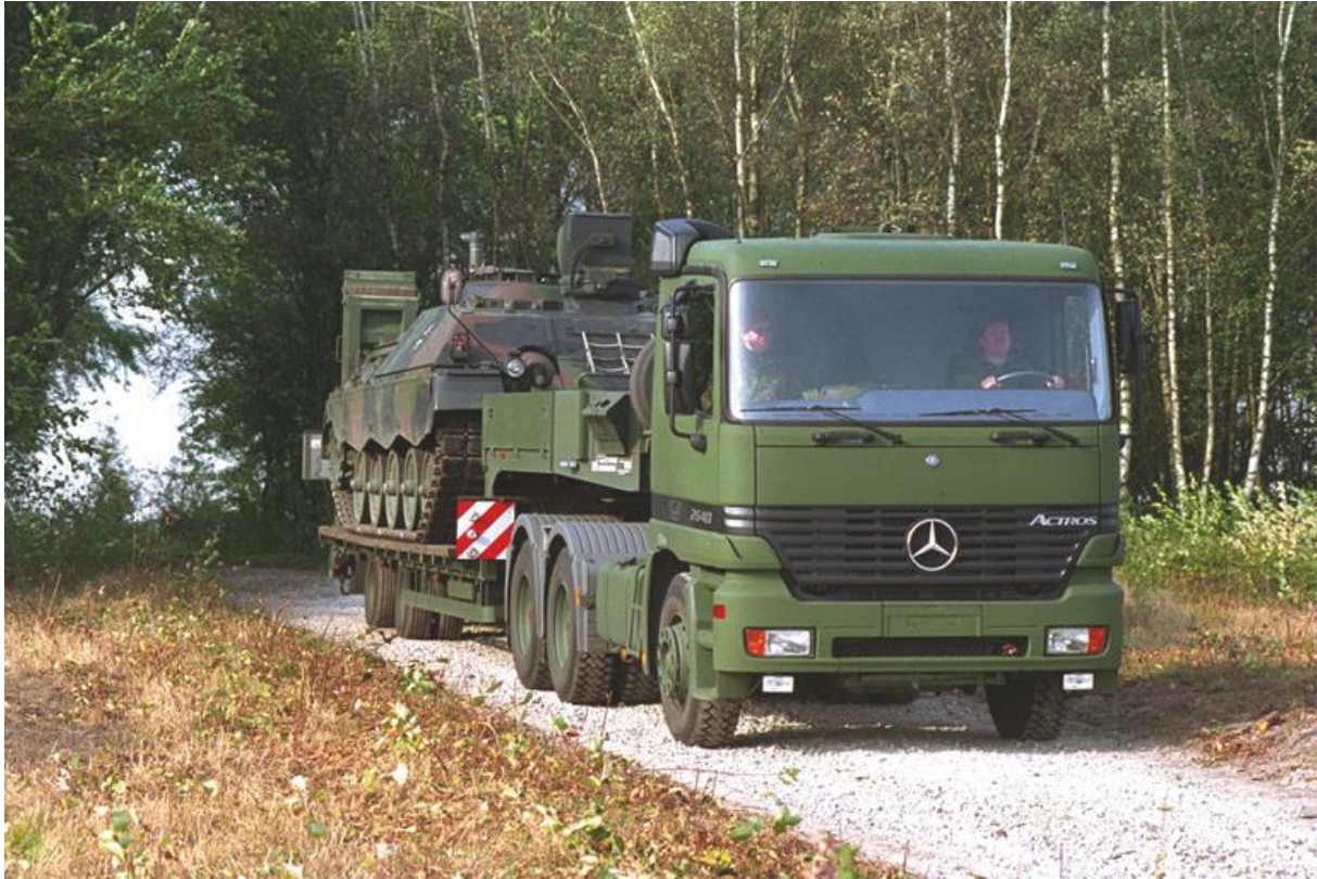
A Mercedes-Benz Actros 2547 tractor truck. Note the exceptional width warning panels in front of the tracked vehicle.
