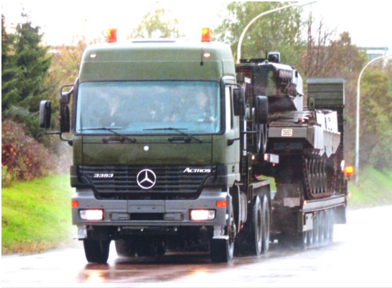
Mercedes-Benz Actros 3353 tractor truck hauling a Leopard 2 MBT on a wet tarmac surface. Modern trailers are in general too small because of compliance requirements set by recent traffic regulations.
