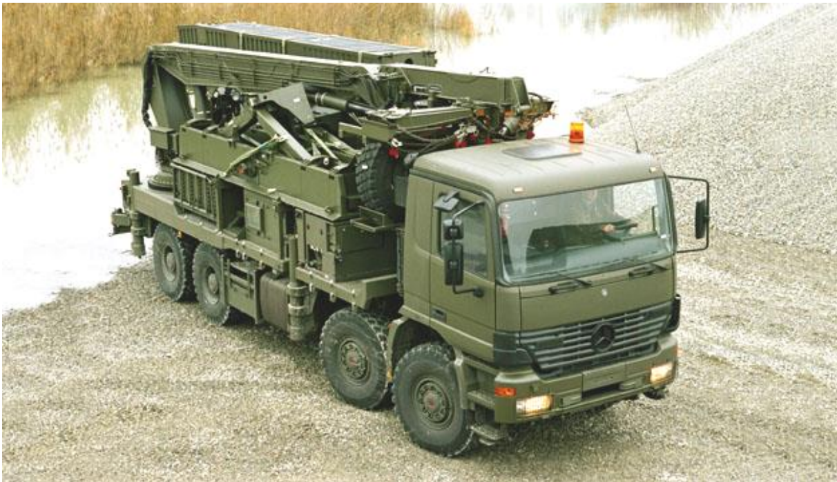
Mercedes-Benz Actros (8x8) with crane hoisting device for the Dornier Eurobridge.
