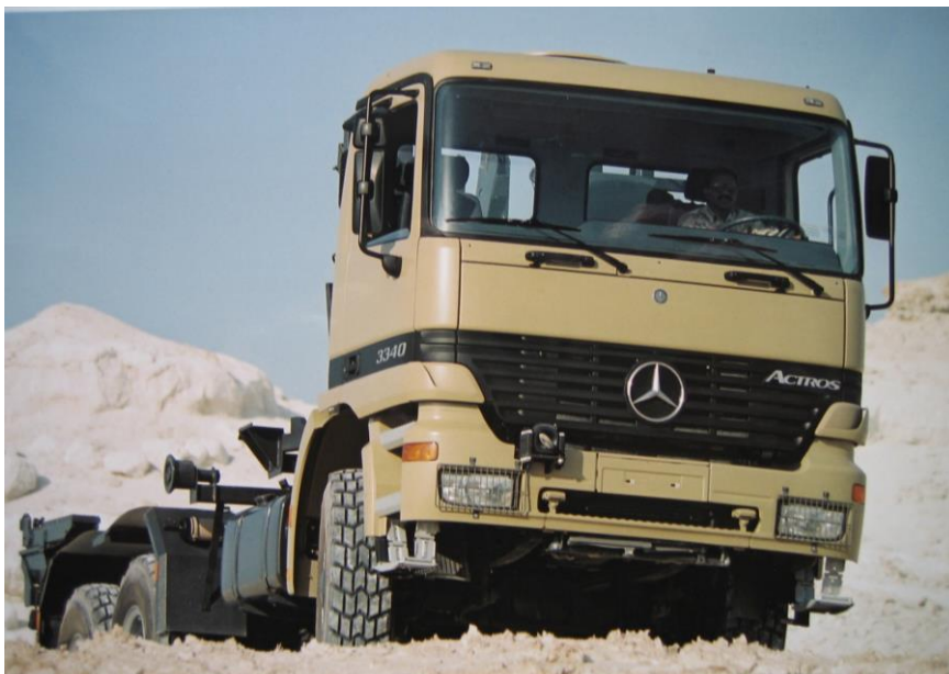
Mercedes-Benz 3340 Actros (6x6) fitted with an empty load handling system. Note the exit box for the rope of the recovery winch at the front.
