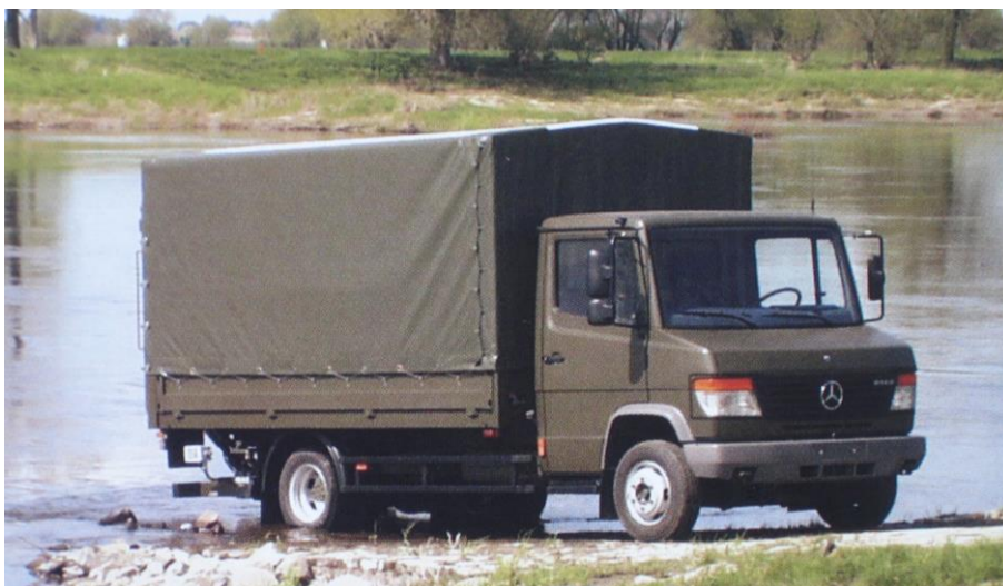
Mercedes-Benz Vario with large rear platform and high tarpaulin arrangement for large-seize loads.
