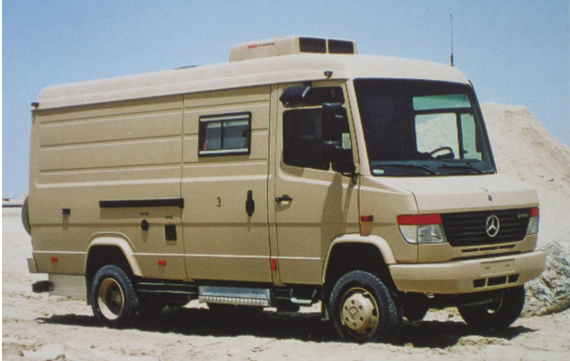
The Mercedes-Benz Vario utility vehicle in sand colour. The All Wheel Drive (AWD) can be recognised by the enhanced ground clearance. An air conditioning system is fitted to the roof of the vehicle. Such agile trucks are well suited for EOD teams for all governmental services if police or the military.
