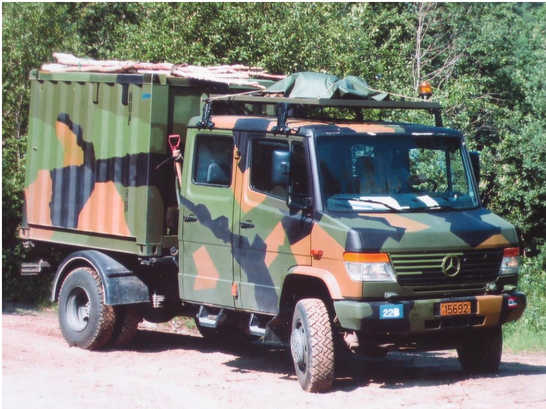
A Mercedes-Benz Vario of the Norwegian Army with extended cab and container platform at the rear. Note the twin rear wheel arrangement.
