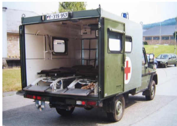
Left: The same vehicle from the rear left side. Note the lifting eyes to deploy the vehicle as a sling load. Ozelot-related vehicles use the more powerful 5-cylinder 4-stroke diesel engine OM 602 DE 29 LA developing 88 kW (119 hp), thus enabling the employment of trailers.
