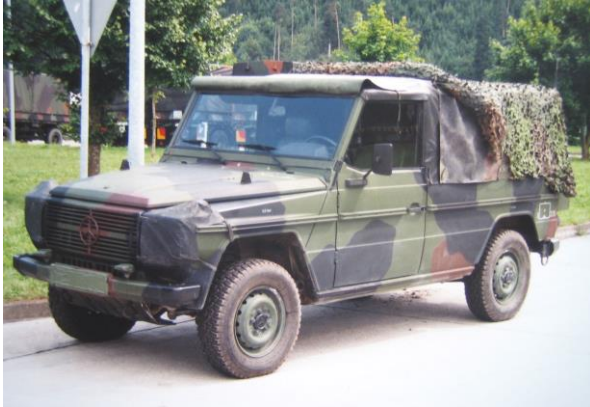
Left: LKW 0,9 to gl (4x4) MB Typ 250 GD long wheelbase (2850 mm), soft top, with equipment set artillery survey team Right: LKW 0,9 to gl (4x4) MB Typ 290 GDT Wolf WSA-2, Maintenance vehicle for LeFlaSys AD system Ozelot.
