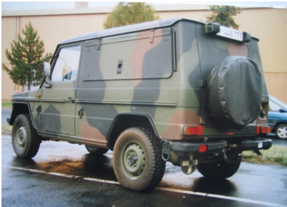
Left: The same vehicle from the rear left side. Note the lifting eyes to deploy the vehicle as a sling load. Ozelot-related vehicles use the more powerful 5-cylinder 4-stroke diesel engine OM 602 DE 29 LA developing 88 kW (119 hp), thus enabling the employment of trailers.
