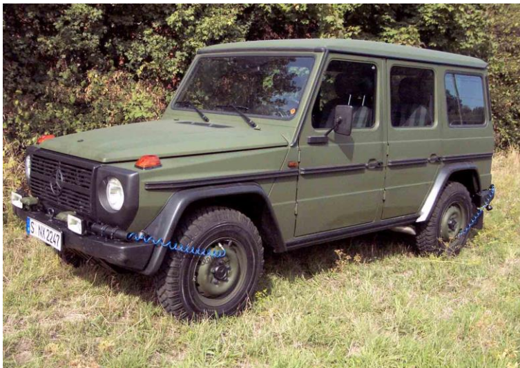
Mercedes-Benz G 270 CDI with additional front grille protection, fitted with radio set and large roof stowage arrangement. Such vehicles went to Scandinavia.
