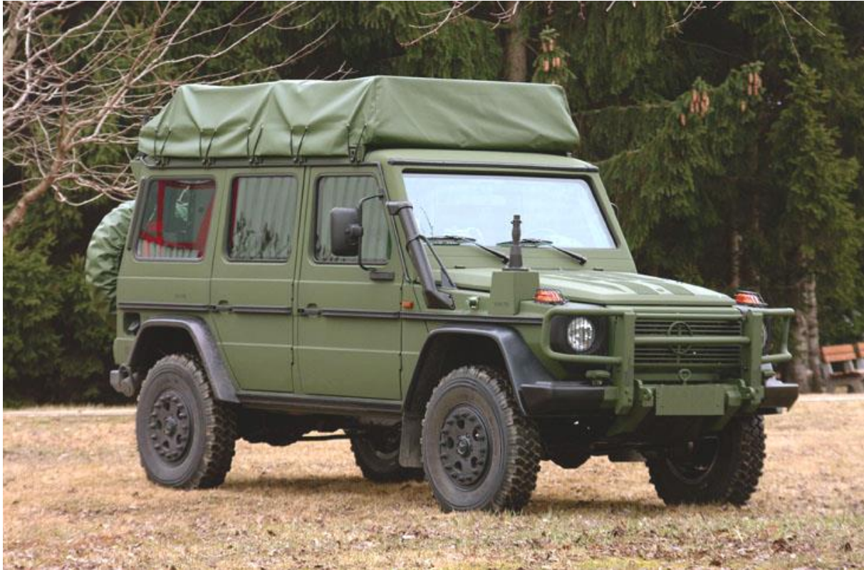
Mercedes-Benz G 270 CDI with additional front grille protection, fitted with radio set and large roof stowage arrangement. Such vehicles went to Scandinavia.
