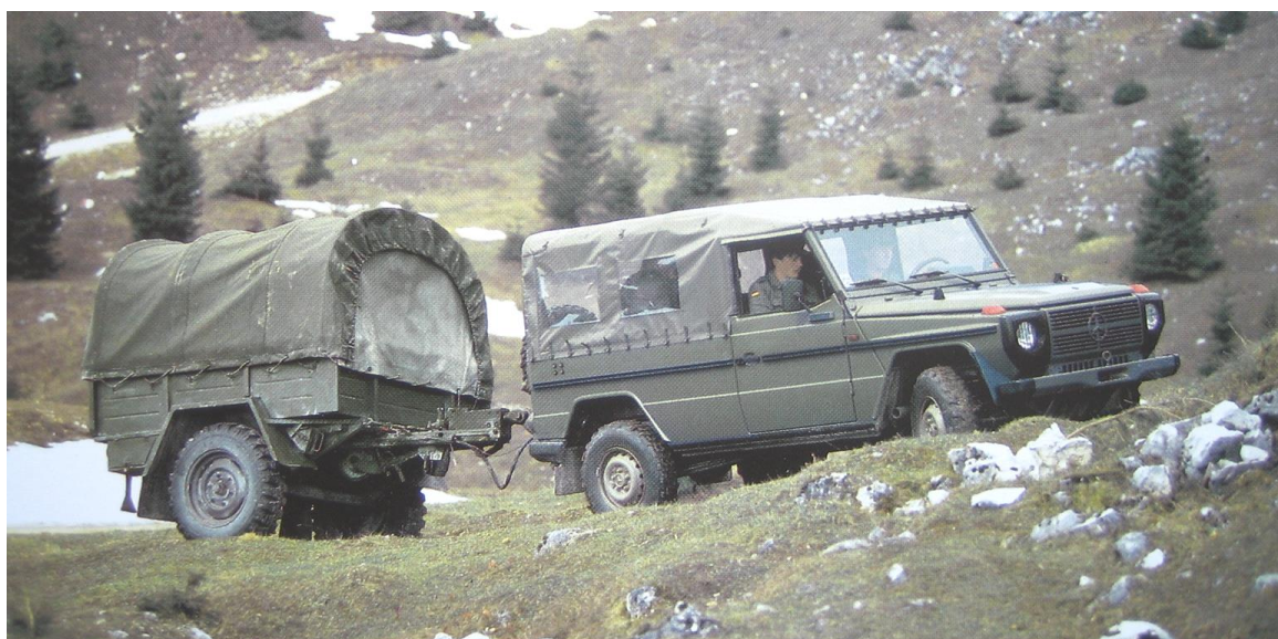
A Mercedes-Benz G-Class B10 variant towing a 1.5-ton trailer of the German Armed Forces.
