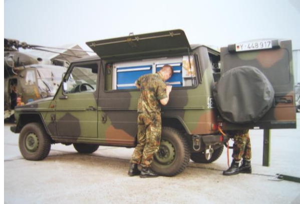
Left: LKW 0,9 to gl (4x4) MB Typ 250 GD long wheelbase (2850 mm), soft top, with equipment set artillery survey team Right: LKW 0,9 to gl (4x4) MB Typ 290 GDT Wolf WSA-2, Maintenance vehicle for LeFlaSys AD system Ozelot.
